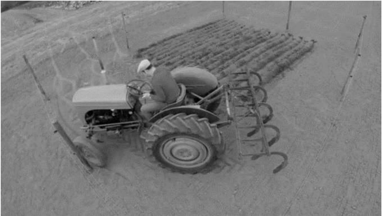
‘Harrowing the Square,’ a demonstration Ferguson used to show how the tractor could operate in any space. The harrow is lifted clear of the ground by the three-point linkage, and the tractor can pivot on the inside wheel.
