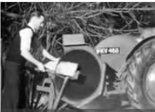
Fitted with a circular saw – and no safety guards!
