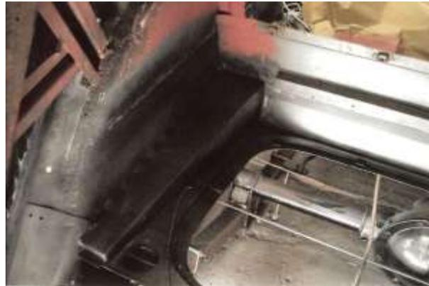
“All the woodwork has been remade and given 3 coats of clear Sadolin. The chassis has been taken down to bare metal, repaired, and then new bushes fitted. It has had 3 coats of Hammerite, and finally Waxoyled inside. All steering, springs, suspension and brakes parts have been given similar treatment.
