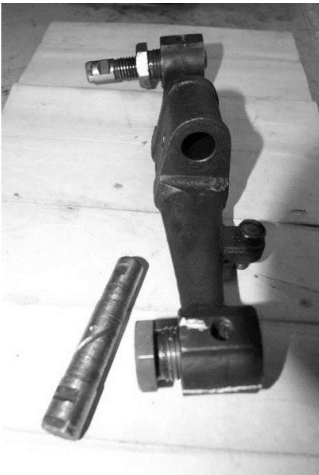
The photo shows the old vertical link with the bushes and fulcrum bolts. It is easy to see how worn the old fulcrum bolt is. The hairline cracks are marked with chalk.
