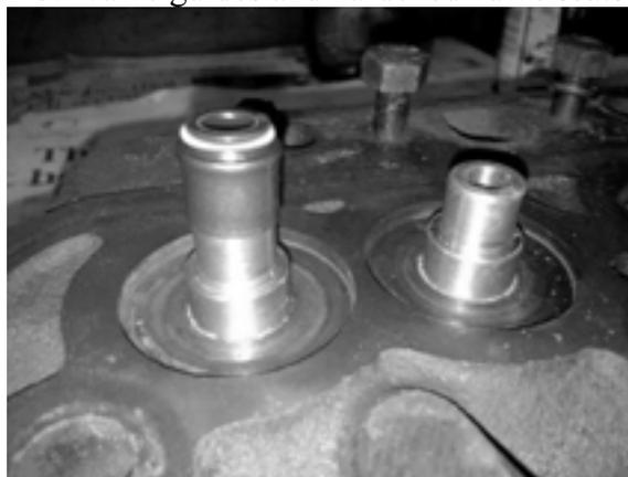
Valve seal in position, ready to press down
