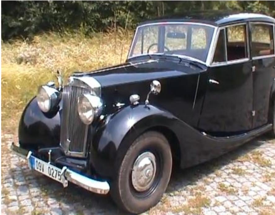
The car appears to be well-preserved, and the driver – or at least the cameraman – has confidence in the brakes, because towards the end of the clip the car draws up quite rapidly to stop just short of the camera. Notice, however, the drooping passenger door-handle: whoever replaced this handle did not realise that the new spindle needs to be twisted through about 20° in order to align it properly.
